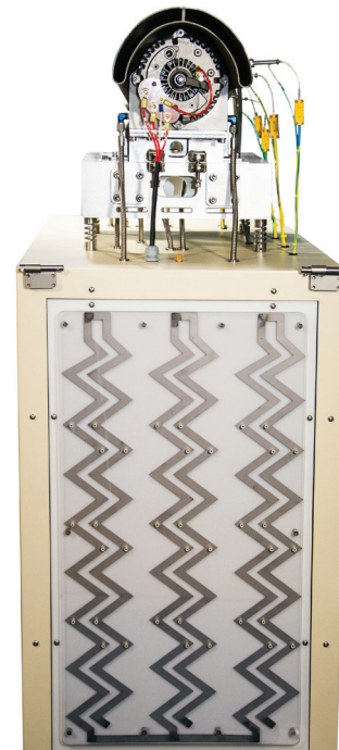
Variable 3-Phase Generator and Resistive Load
